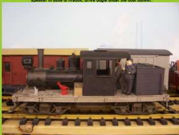
8 AA cells, EBC and direction servo, all in bunker to create best traction. Now it sounds like the workhorse it really is, fast beat exhaust, yet slow and surprisingly strong.
