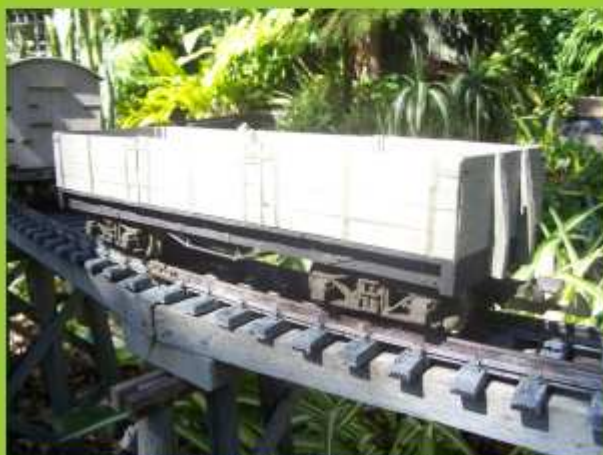
This HJ Class is one of Geoff's "convertible" wagons. The basis is a set of Flat oars, on which various body shells can be fitted.
