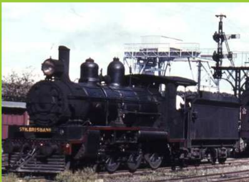
A PB15, 1924 version [Walschaerts Valve Gear] steam loco.
