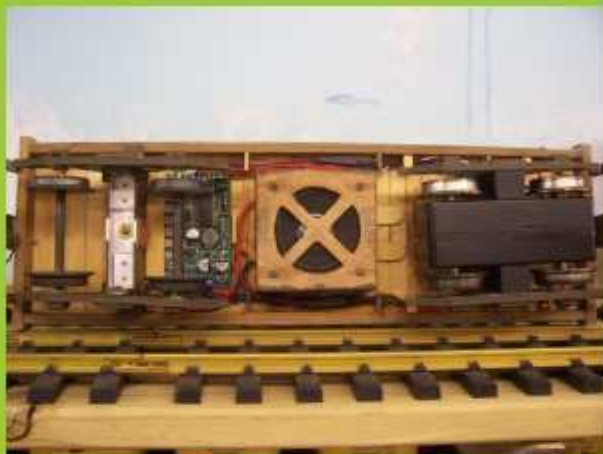
The underside of this loco, sound board under leading bogie. Speaker in base of firebox, drive bogie under the coal bunker.
