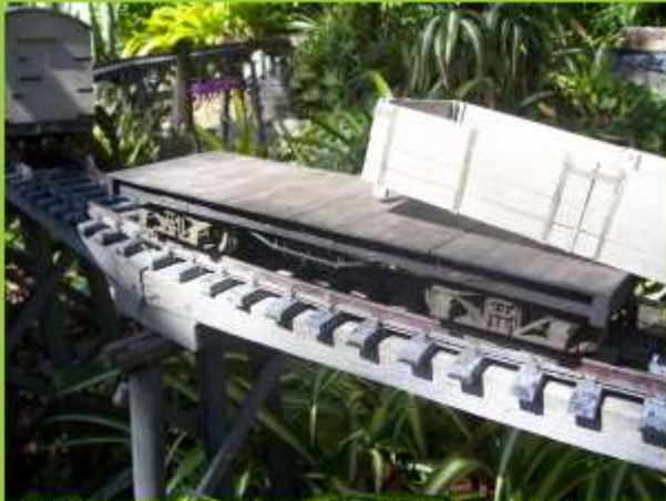
Here we see the four plank side & end unit removed ready to accept a different body shell.
